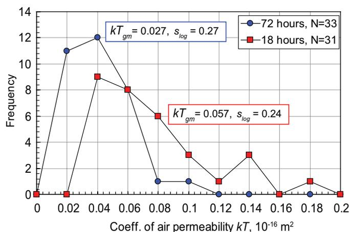
Fig. 6: Frequency distribution and statistical parameters of test results
