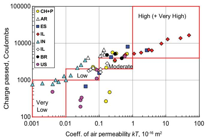
Fig. 8: Comparison of charge passed per ASTM C1202 and  $kT$  values per SIA 262/1-E,<sup>9</sup> from Reference 8. The data were taken from numerous sources. Permeability classes for the two test standards are also shown
