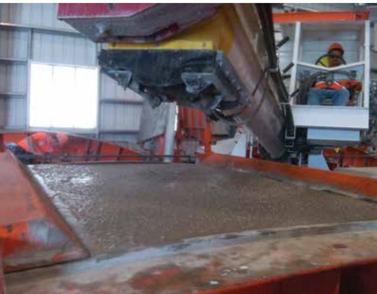
Fig. 2: Concrete was transported to each form using a vehicle equipped with a hopper and an auger. During and after filling, the steel form was vibrated for a total of 8 minutes to consolidate the mixture
